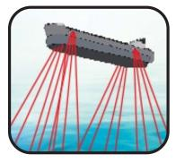
In **taut-leg** configurations, MoorSafe precisely calculates anchor line angulation by detecting even very small variations in angle, providing accurate and immediate alerts for changes in mooring line behavior.
